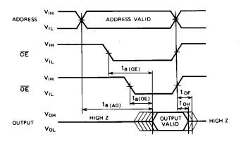
Test conditions for A.C. characteristics Input voltage:  $V_{IL} = 0.45V$ ,  $V_{IH} = 2.4V$  Input rise and fall times:  $\leq 10$ ns Reference voltage at timing measurement: 1,5V
