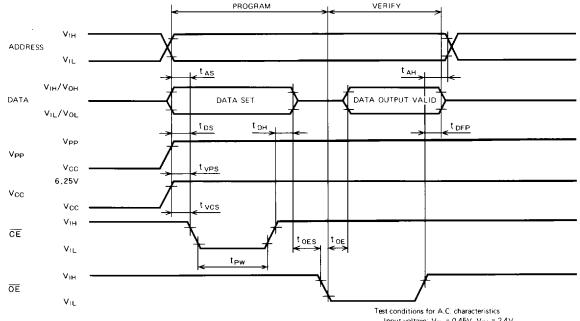
Input voltage:  $V_{|L} = 0.45$ ,  $V_{|H} = 2.4$ V Input rise and fall times:  $\leq 20$ ns Reference voltage at timing measurement: Input, Output "L" = 0.8W. "H" = 2V.
