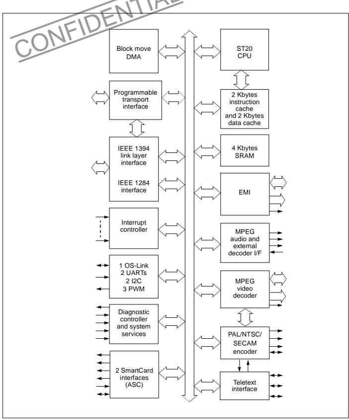
Figure 2 STi5512 architecture block diagram
