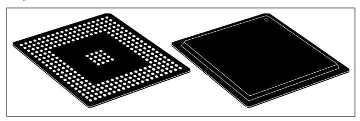
Figure 5 256-pin BGA package
